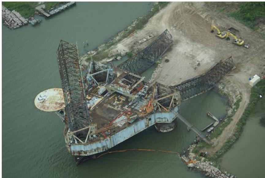
**Fig. 11.** The dead-stacked jackup rig *Zeus*, being dismantled in the Freeport Ship Channel.
